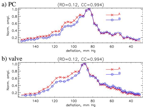
Figure 12: Comparison of normalised waveforms obtained from pressure measurements in the cuff (A) and from the low frequency part of the microphone data (B) when the cuff is deflated through a) the feedback loop in the PC and b) the valve.
