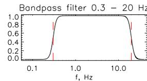
Figure 4: Butterworth bandpass (0.3–20 Hz) filter of 6<sup>th</sup> order.
